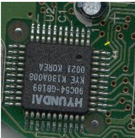
Figure 6. Cut Here to Disable the DO (data out) line.
